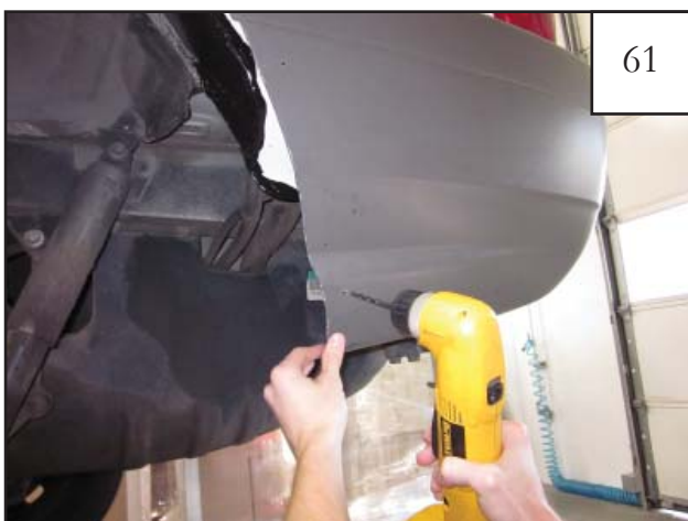
61 Using a 3/16" drill bit, drill the two holes marked in step 60.
