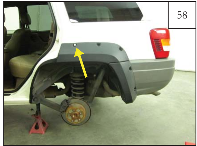
58 Install one screw (SW1-0045) in top front hole of flare to hold it in place while making marks in the next step.
