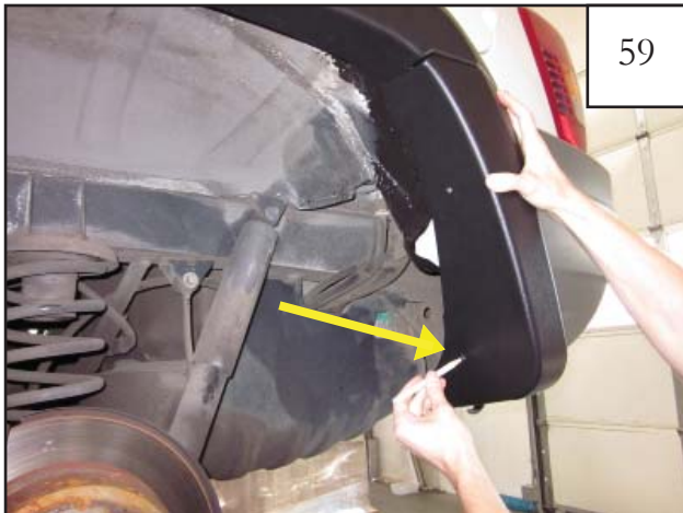
59 Hold flare and bumper piece in place so that the holes in the bumper piece barely overlap the cut bumper and mark the locations on the edge of the bumper. Use an awl if needed (2 locations).
