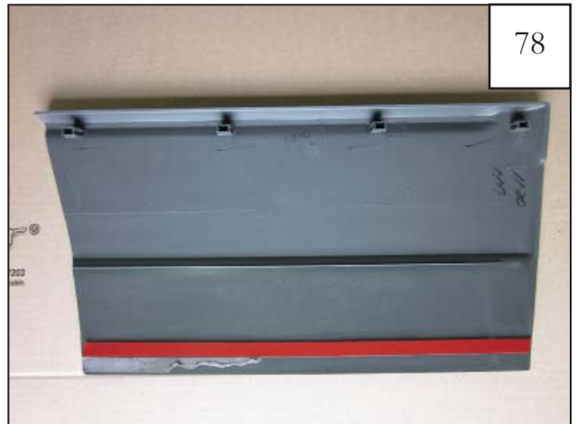
Apply supplied double sided tape (MT1-0025) to plastic where primer was applied in previous step.
