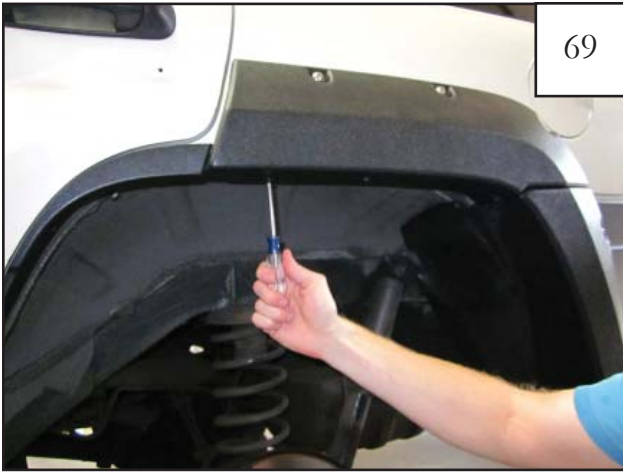
Secure flare to fender with panhead screw (SW1-0056) through holes drilled in step 68.
