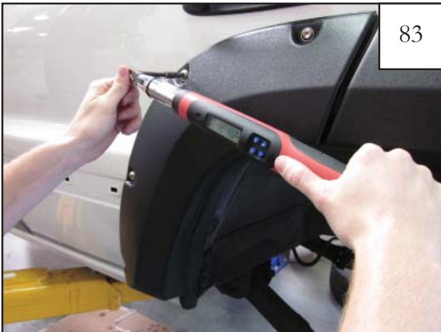
Once all screws have been started, snug screws to vehicle. Torque screws to 24 in•lb (2 ft•lb). DO NOT OVERTIGHTEN!
