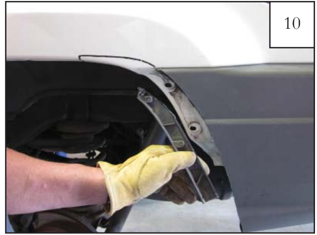
Remove trimmed bumper support bracket.
