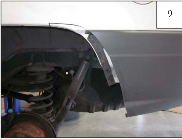
Use a cutoff wheel to trim the bumper support bracket parallel to trimmed bumper.
