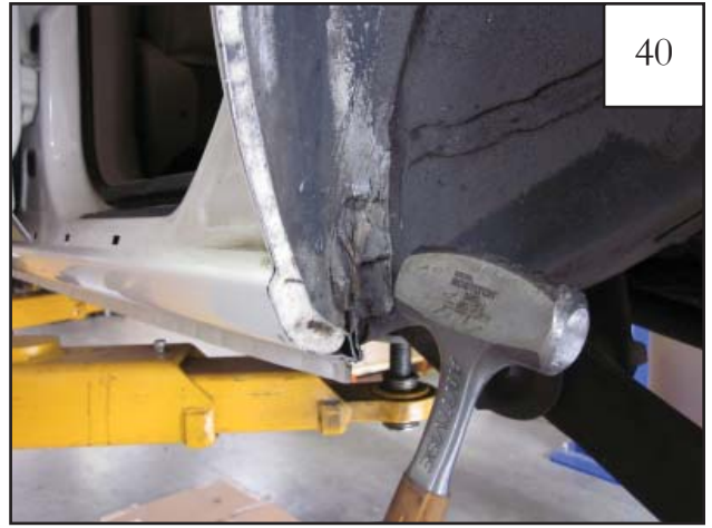
Using a hammer, flatten pinch weld tabs against inner wheel well.
