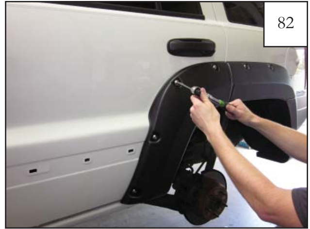
Hold flare in place on fender. Using the provided torx bit driver and ratchet with 3" extension, start each screw into drilled holes.
