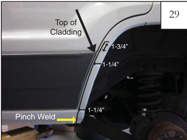
Mark vehicle for cutting: Make a line 1-1/4" in from the edge of the wheel well extending up from the bottom pinch weld to 1-3/4" above the top of the cladding.
