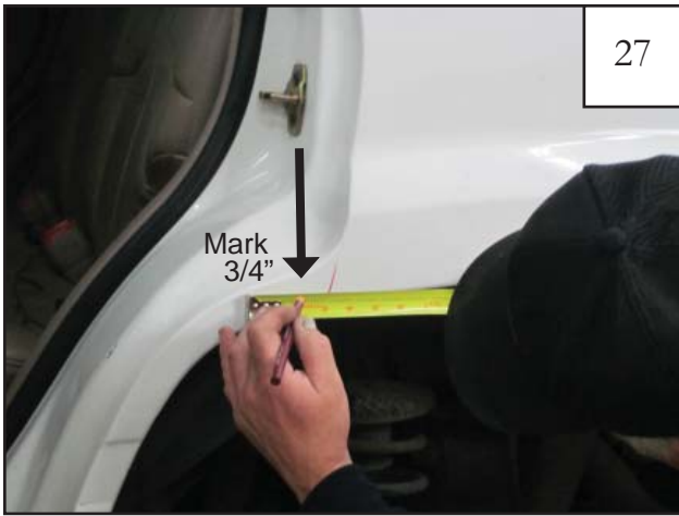
Measure 3/4" toward the front of the vehicle from the mark made in previous step along fender lip. Using a grease pencil, make a mark.
