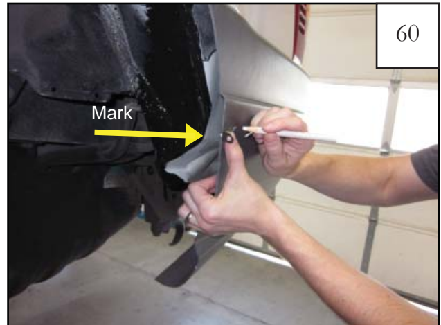
60 Mark Hold mounting bracket (MB1-0003) in line with mark made in step 59 and make a mark through the hole location in the bracket. Repeat for second bracket.
