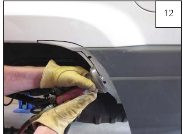
Using a cut off wheel or other suitable tool, cut along line marked in step 11 removing the inner flange.
