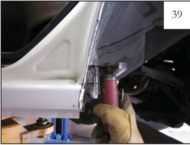
Using a cut off wheel or other suitable tool, cut along horizontal marks made in step 37.
